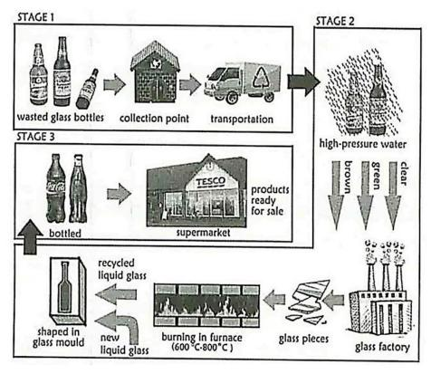
The procedure for reusing bottles made of glass is depicted in the diagram. Overall, there are a number of steps divided into 3 stages, commencing with empty bottles and finishing with these filled with commercial products on sale at retail outlets.
